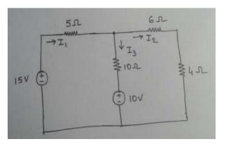
b) Use the nodal analysis to determine the current through R<sub>3</sub> of the following circuit.
